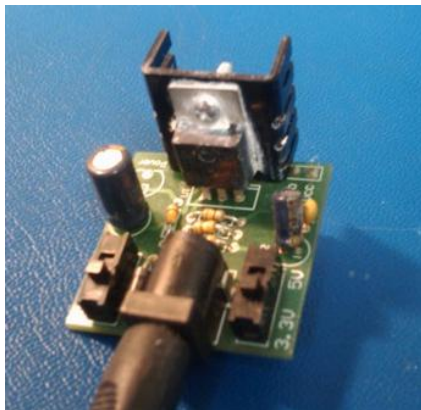
Figure 2.1: A heat Sink Attached to a Linear Regulator (Content are acquired through All-Battery.com)
