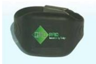
Figure 4.9: 2.45 GHz Active RFID Wristband Tag (Source from gaorfid.com)
